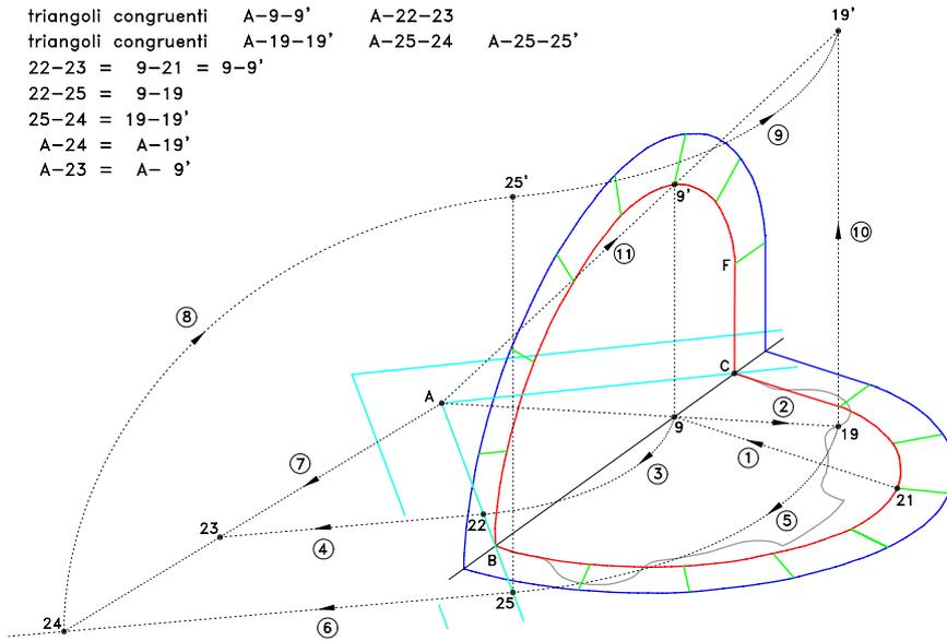
Figure 6 (top left). Axonometry illustrating the method used by Delorme to trace the height of the vault, starting from the plan (in grey) and from a vertical section of the vault itself turned onto the horizontal plane. The image shown here reproduces the bi-dimensional geometrical operations used by Delorme himself in his study (see figure 2). The section of the intrados is shown in red; the extrados in blue; the conjunctions between the ashlar in green.
