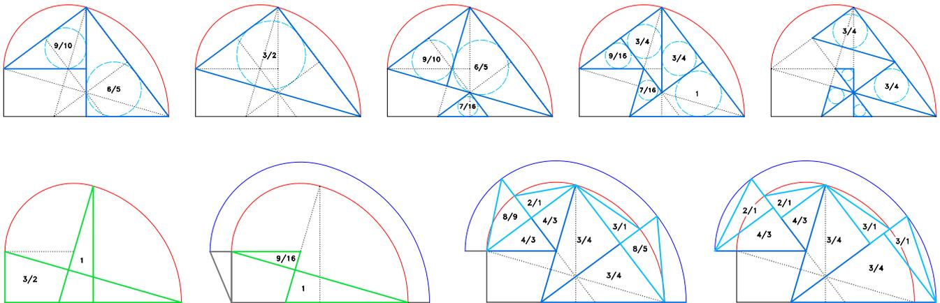
They therefore define the limits of the figure of construction and therefore the shape of the inferior surfaces, the intrados of the rampant vault.<sup>12</sup>
