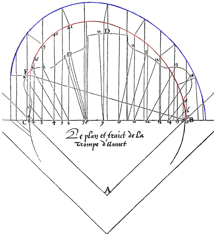
Figure 3 (top left). Delorme, *op. cit.*, f. 96v. Trait used for the construction of the development boards of the trompe of Anet. The ovals obtained by means of the construction presented in the article are highlighted to allow comparison. In the Delorme treatise all diagrams are to the same scale.
